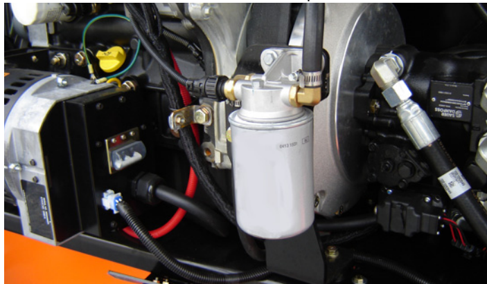
C. Brandstoffilter - Deutz TD2.9 (op motor)
